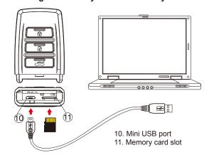
Remove the rear cover of the device, plug the micro USB end of cable into (10) and plug the other end into the computer or other USB power source. After charging is complete, insert the memory card into (11). Then the device will be ready for further operations.
