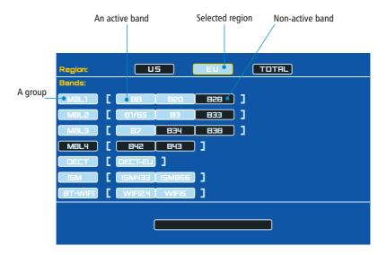
**Move the joystick** in order to go left, right, up, down or press it in order to activate or deactivate certain items. To exit, press the **BACK** button.
