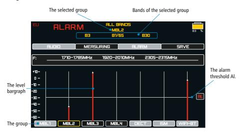
The groups will be displayed at the bottom of the screen. The signal levels by groups are displayed on the bargraphs. By pressing **the joystick to the left and right**, the user can choose a group and see which bands belong to it.
