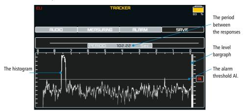
**The alarm threshold** can be adjusted, and the **ALARM** and **AUDIO** functions can be switched on. A subsequent **pressing of the joystick button** selects the ALL BANDS mode.
